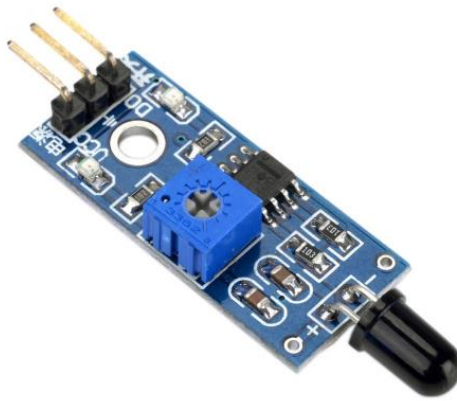
Figure 20: IR Fire Sensor
